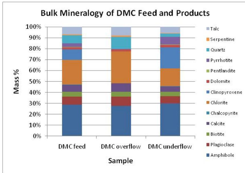
**Figure 5** Recalculated bulk mineralogy for the DMC feed, overflow and underflow
