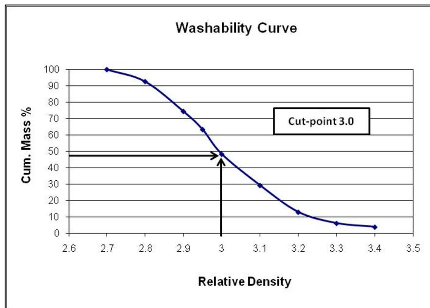
Figure 2 Washability curve (left) and grade and recovery curves for Ni and Cu (right)
