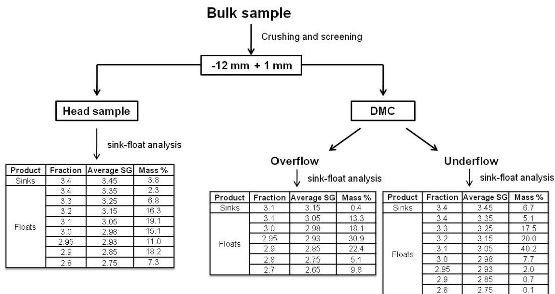
**Figure 1** Derivation of samples for mineralogical analysis
