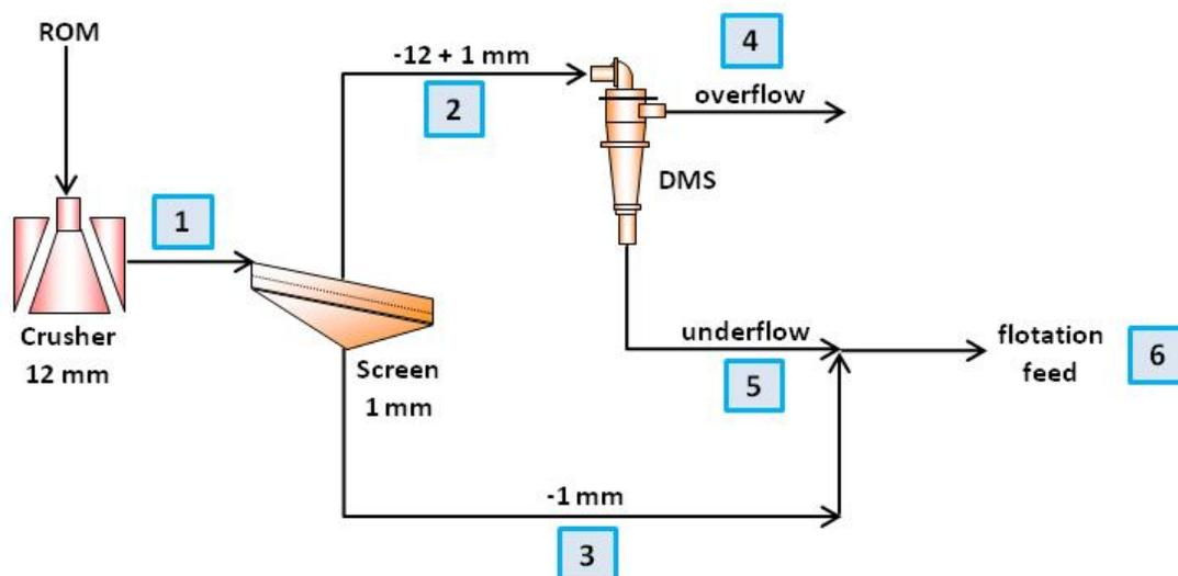
**Figure 4** Flowsheet for the testwork showing different streams
