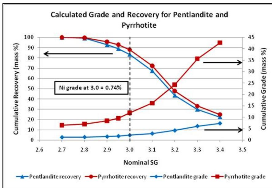
**Figure 3** Cumulative grade and recovery curves calculated for pyrrhotite and pentlandite from the sink-float analysis
