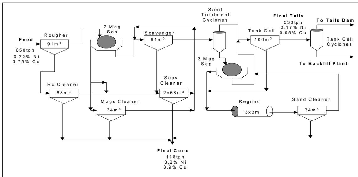
Figure 2a. Flowsheet with four separate cleaner banks
