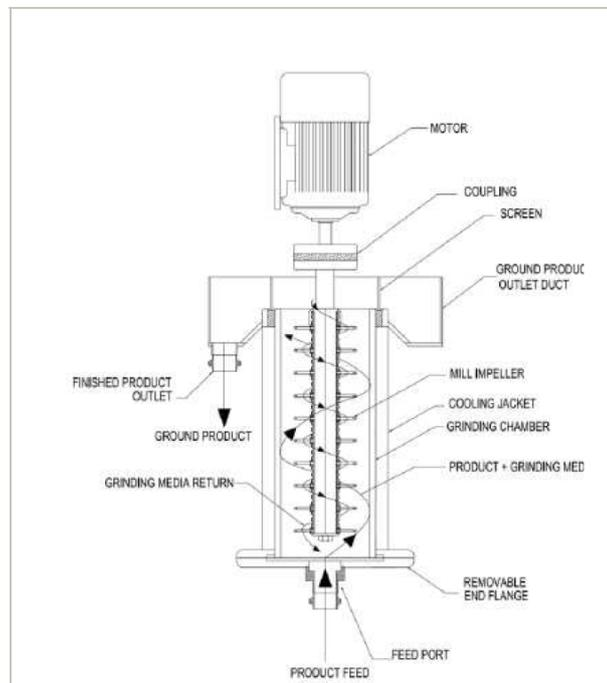
Figure 4: High speed vertical mill (Sverak, 2007)
