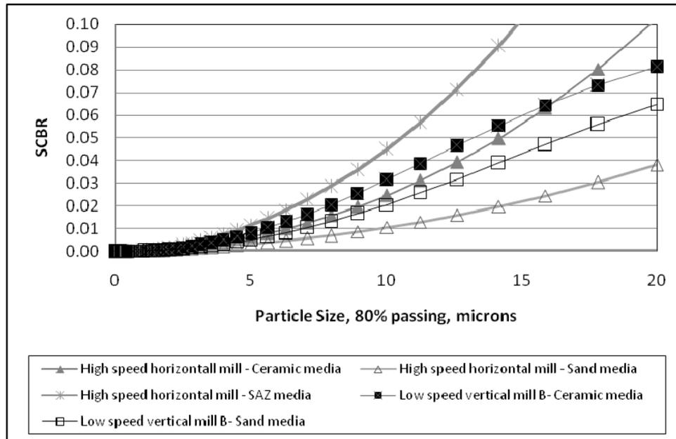
Figure 6: Specific cumulative breakage rates using seasoned sand, ceramic and SAZ grinding media.
