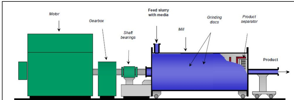
Figure 1: High speed horizontal stirred mill (2009).
