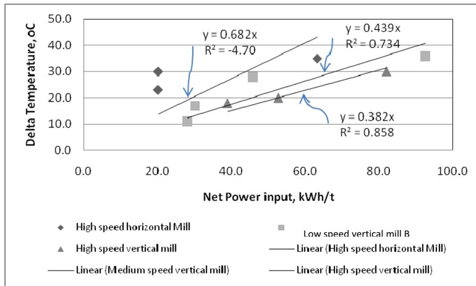
Figure 8: Temperature increase per specific energy input.
