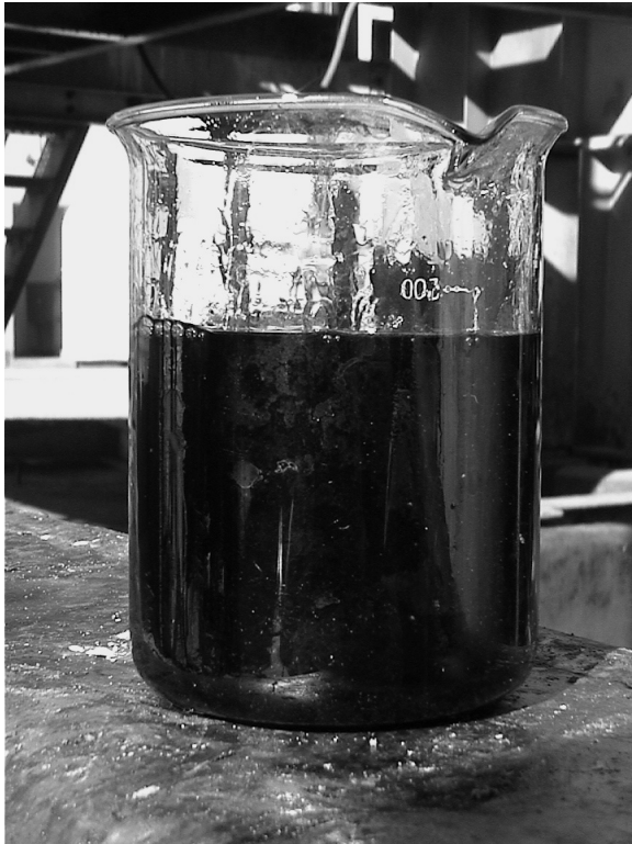
Figure 7: BMMS Tricanter centrifuge organic discharge.
