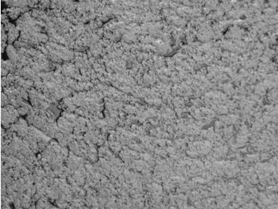
Figure 4: Crud 'cake' discharged from filter press
