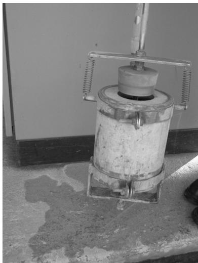
Figure 5: Air Hold Up (AHU) device
