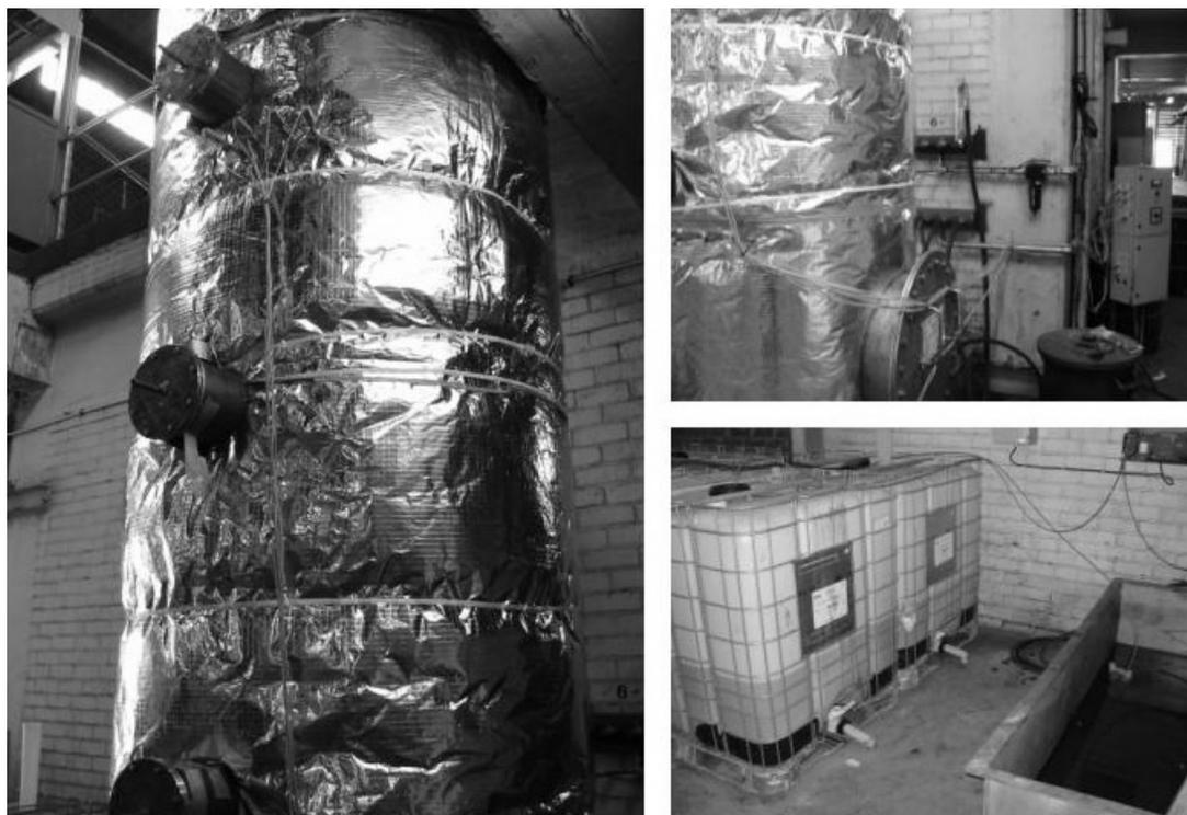
**Figure 6:** Photographs of the Large Diameter Column with peripherals at the Exxaro Pilot Plant showing the sample ports on the left, electronics and manhole right top and on- and off-solutions right bottom.
