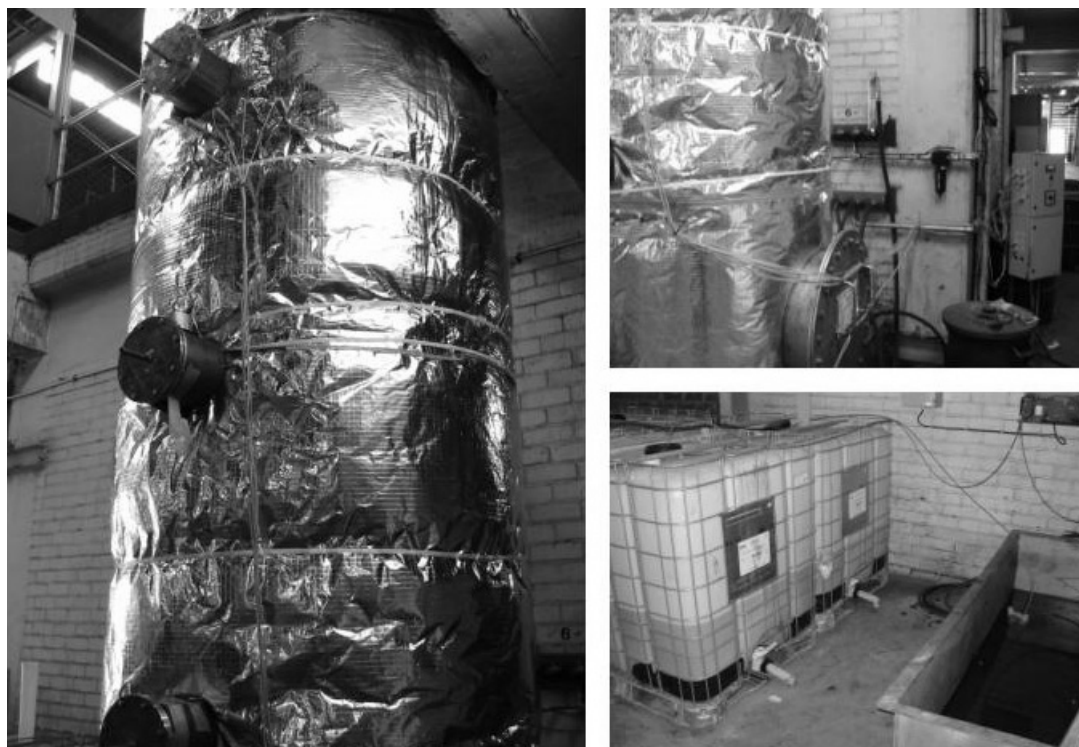
Figure 6: Photographs of the Large Diameter Column with peripherals at the Exxaro Pilot Plant showing the sample ports on the left, electronics and manhole right top and on- and off-solutions right bottom.
