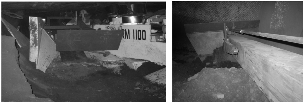
Figure 8. Scoop used to load cut rock onto the belt conveyor
