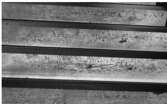
Figure 1. Typical misalignment damage on a girth gear
