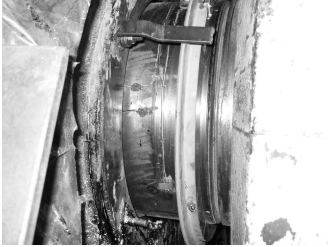
Figure 5. Tufnol disk mounted on the mill pinion next to the gear teeth
