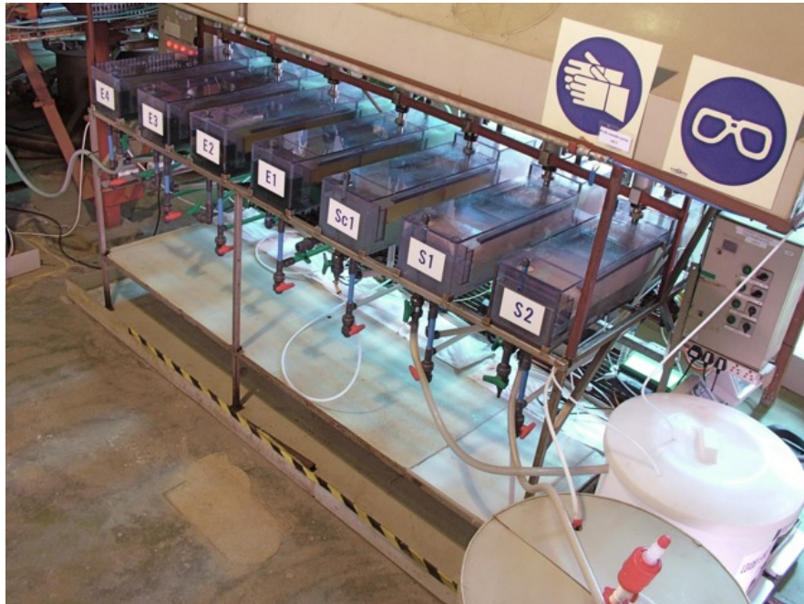
Figure 1. Front view of pilot plant, showing mixer settlers and stripped organic holding tank and the loaded strip liquor tank on right.
